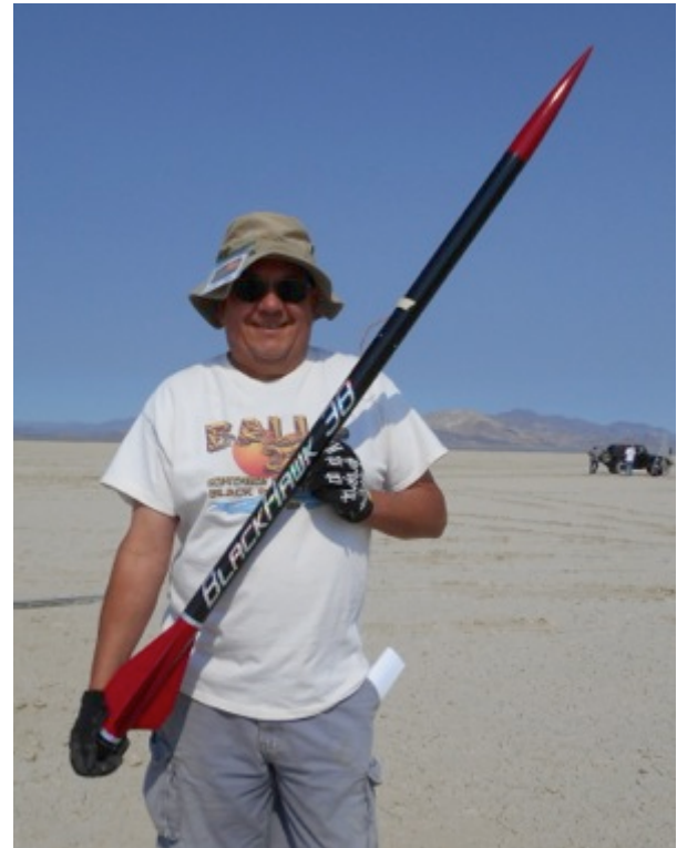
At left is Bill Good Sr. with his minimum sized rocket, which won the best looking and lightest weight awards, unfortunately it went unstable because of a motor case burn through at the nozzle and crashed near the pads.
