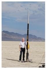
Former TRA President, Ken Good proved that the third time is the charm when he managed to get his Drake 2 rocket (left) flown successfully. The Drake features electronically staged motors, but not in the conventional method. When the first motor burns out, it is ejected from the airframe and a second motor slides into the first motors place and is ignited. He
