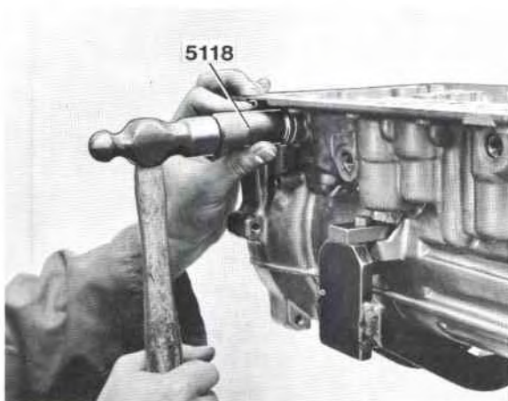
5118* Drift for fitting control shaft sealing ring
