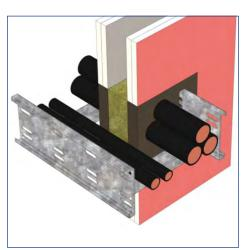
FS709 Intumastic HP direct in drywall opening with various service penetration: El120
