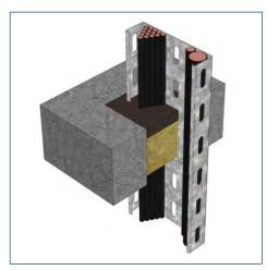
FS709 Intumastic HP direct in concrete floor opening with cable tray & cables: El120
