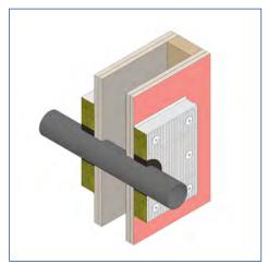
FB750 double batt pattress fit + FS709 Intumastic HP seal: EI120
