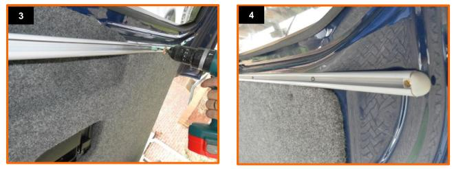
The top track must be fitted so the holes are drilled upwards (if the tailgate is closed) to avoid damage. (fig.5 & 6 shows tailgate open)
