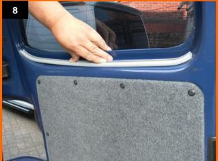
2. Start by using one of the pre-drilled holes in the track as a guide, drill a hole into the window surround and screw the track into place. (fig.9 & 10)
