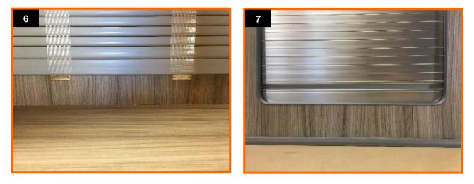
The door can be fitted to operate in a vertical or horizontal direction. If the door is to operate sideways (horizontally) in a vehicle then apply the supplied magnetic tape to the edge of the door so it connects to the Metal Angle Plates. This helps to keep the door closed whilst travelling.
