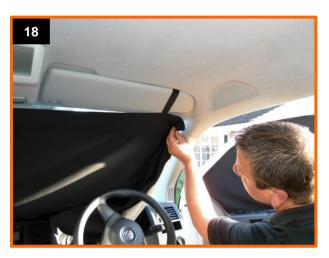
4. Fold down one sun visor whilst holding the middle of the blind up in place. (fig.19 & 20)
