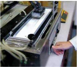
The Scrub Test evaluates the resistance of the coating to repeated cleaning and is measured by the following method:
